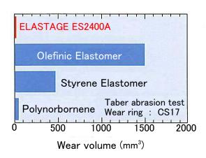
**Test method**JISK6264 1 kg Load, After the 1000 revolution
